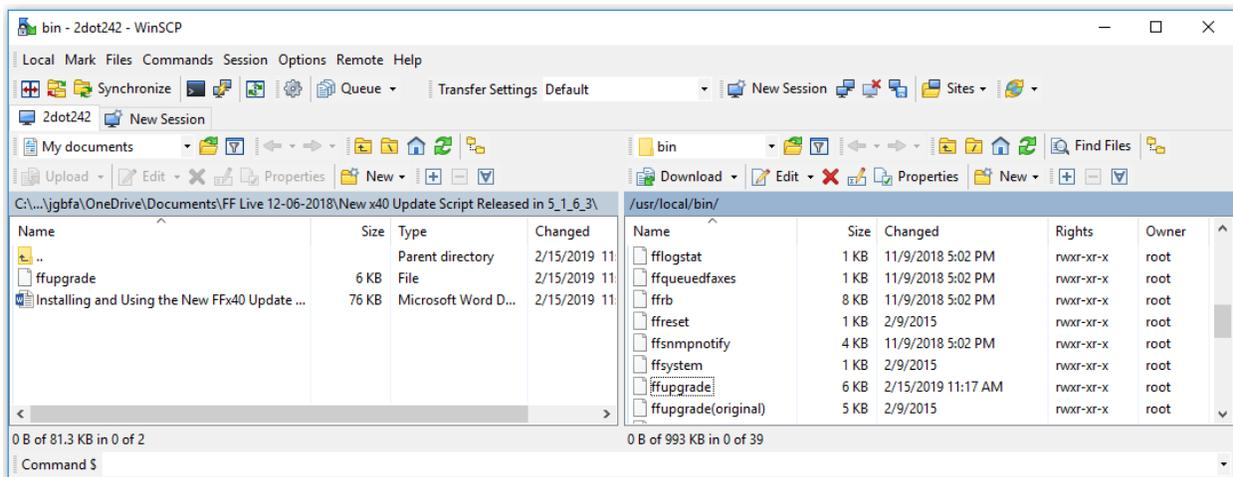
The above screen shot shows the new ffupgrade file with the correct attributes set (under the “Rights column). With that in place you can disconnect the SCP connection.
