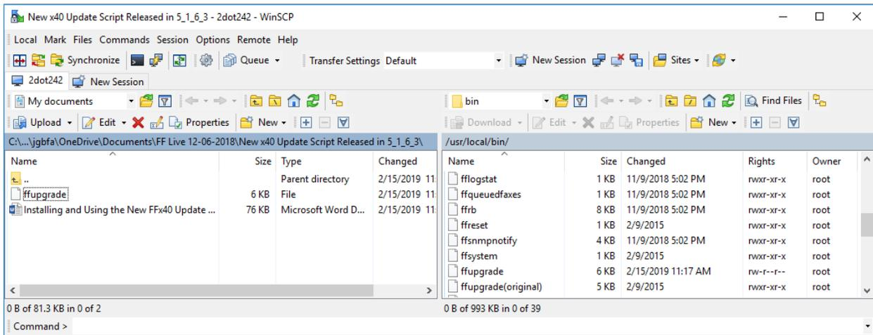
The above screen shot shows the new version copied in (note that the file size of the new script is slightly larger than the older script, right click on the file and bring up properties to see exact byte size). The file needs to be 5519 bytes in size. Also note that the file does not have executable (lower case x) “rights”.
