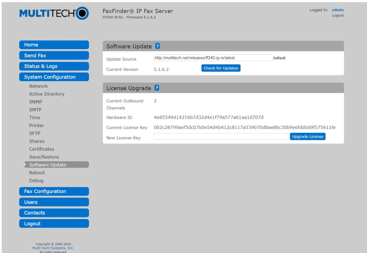
The above screen shot shows the update source (path) for the FF240-IP.Rx models after clicking on "default". Software versions 5.1.6.2 and older default the path to look in the "latest" folder on multitech.net.
